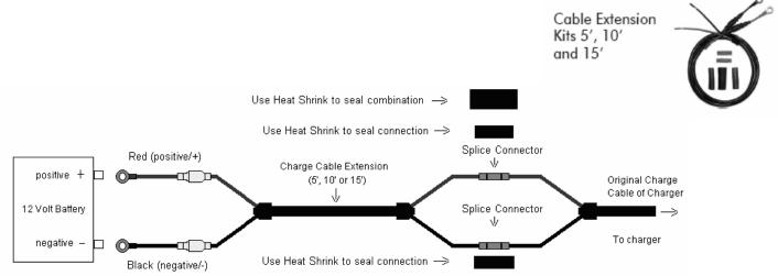
To connect the charger to the battery (batteries), route your charge cables from the charger to the batteries, being cautious to avoid sharp objects, and use the supplied wire ties to hold them securely and neatly in place.
