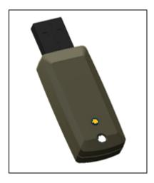
The USB connector without its cap is to the upper left. The small button activates a read cycle when pressed. The round aperture allows light from the chargers Green LED to enter the unit and be received on the surface of the PIN photodiode.
