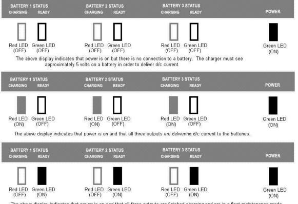
The above display indicates that power is on and that all three outputs are finished charging and are in a float maintenance mode.
